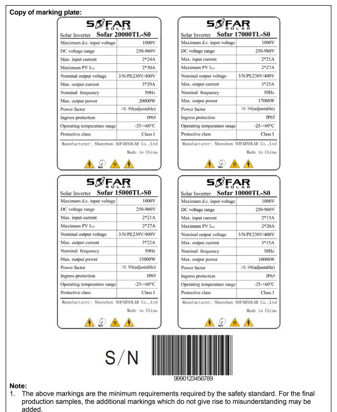
2. Label is attached on the side surface of enclosure and visible after installation.
